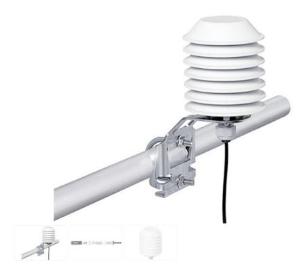
The compact, long-term stability weather sensor OTT TRH is responsible for the measurement of relative humidity and temperature. In addition it can calculate the values for absolute humidity, dew point and mixing ratio and output these via the SDI-12 interface. A protective cap prevents dust and dirt from entering the sensor system. The included protective housing provides weather and radiation protection.
