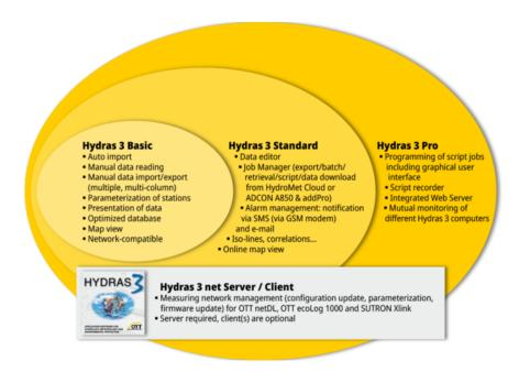
OTT Hydras 3 Basic communication software is a convenient and user-friendly solution for the configuration of OTT dataloggers, for downloading measured values using a notebook, and for automatic remote data collection via modem. Hydras 3 Basic is equipped with a multitude of functions to simplify the setting up of sensors and the maintenance of measurement stations.
