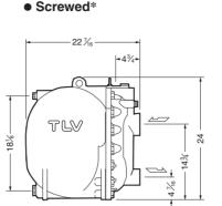
Weight (lb): 273 (Cast Iron), 300 (Cast Steel) \* NPT, other standards available
