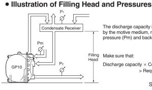
The discharge capacity is determined by the motive medium, motive medium pressure (Pm) and back pressure (P2).
