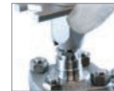
Adjusting the valve aperture
