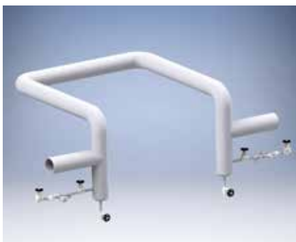
FIG. 14. Bi-directional steam flow requires condensate collecting legs/CDLs on both sides of an expansion loop.
