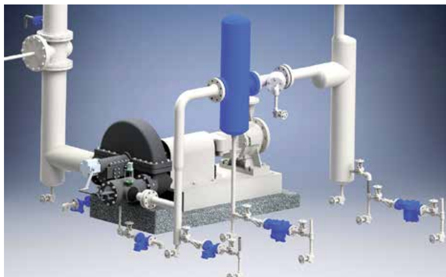
FIG. 16. CCBs may be helpful on a variety of installations experiencing condensate difficulties.
