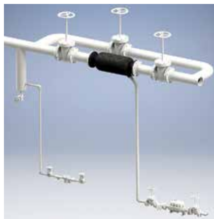
FIG. 15. An oversized collecting leg, a CCB, can help remove larger condensate accumulations.
