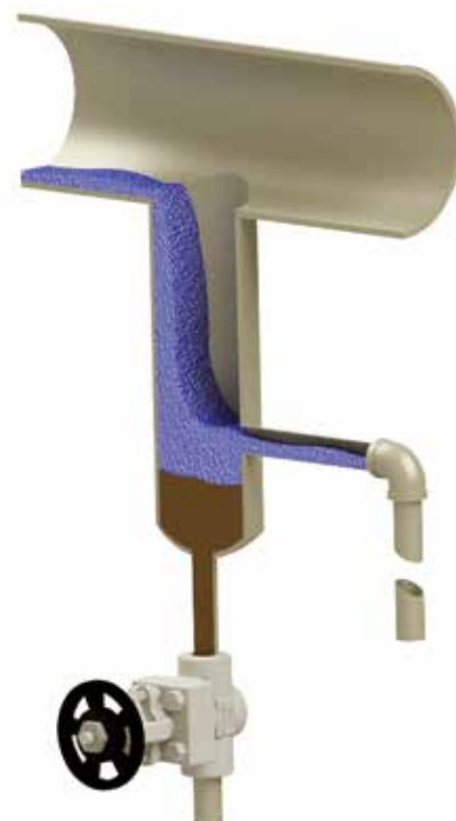
FIG. 2. Collecting legs are wide to catch condensate, deep with a low take-off to hold condensate, and use a mud leg for blowdown.
