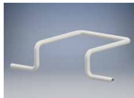
FIG. 10. Danger: Expansion loops on steam lines without a collecting leg to remove condensate can expect water hammer.
