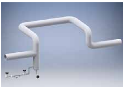
FIG. 13. Uni-directional steam flow requires a condensate collecting leg/CDL on the upstream side of an expansion loop.
