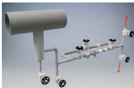
FIG. 8. An effective collecting leg/CDL includes a variety of piping components.
