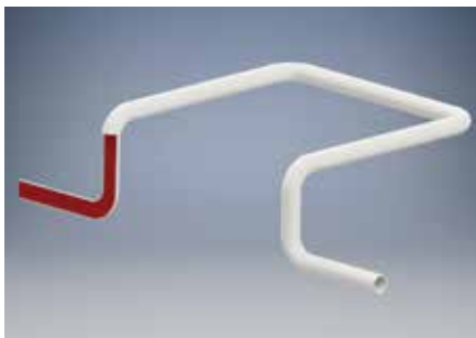
FIG. 11. Danger: Piping designers sometimes believe steam lines have steam flow only within, especially on superheat.
