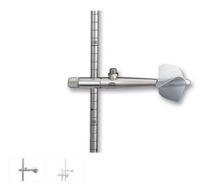
The OTT C2 small current meter for discharge measurements for shallow waters in small rivers, channels, laboratories and river models. Proven a thousand times to measure reliably flow velocities from 0.025 up to 5 m/s. Available for rod measurements on 9 mm or 20 mm rod.
