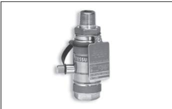
This durable, explosion proof Pressure Switch is used to signal that a deluge valve has opened. It can be specified on a new valve or easily retrofitted to an existing valve in the field.
