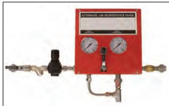
The Automatic Air Maintenance Panel automatically maintains the air or nitrogen pressure within preset limits in a dry pipe sprinkler system or a dry pilot line which actuate Deluge or Pre-action system.
