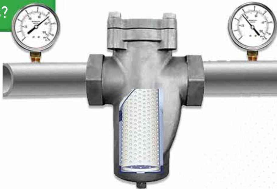
The above image shows two gauges used to detect if a basket strainer needs to be cleaned. In this illustration, the operator has to subtract the pressure of one gauge from the other.
