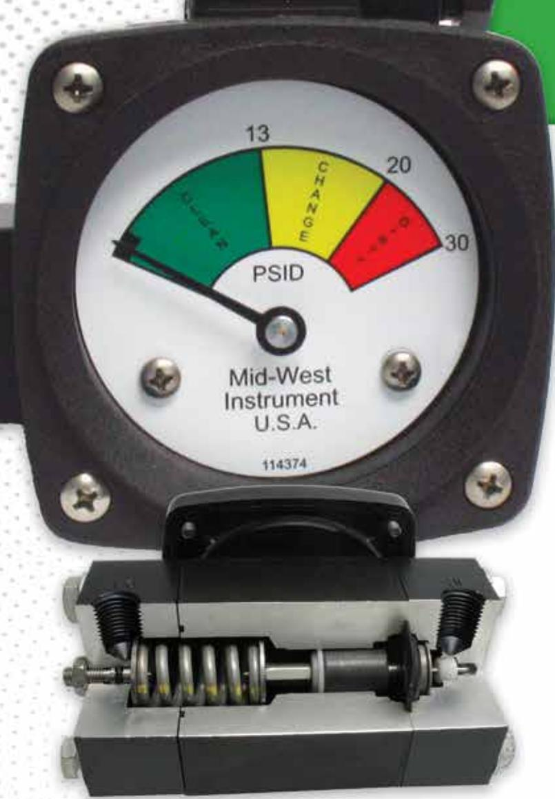
The diaphragm type gauge is very versatile making it the ideal choice for many applications. The diaphragm forms a tight barrier between the high and low ports which allows the gauge to measure pressure differences between dissimilar process fluids. Diaphragm gauges work well with higher temperatures and “dirty” fluids. Diaphragm gauges feature +/- 3-2-3% and 5% accuracy.
