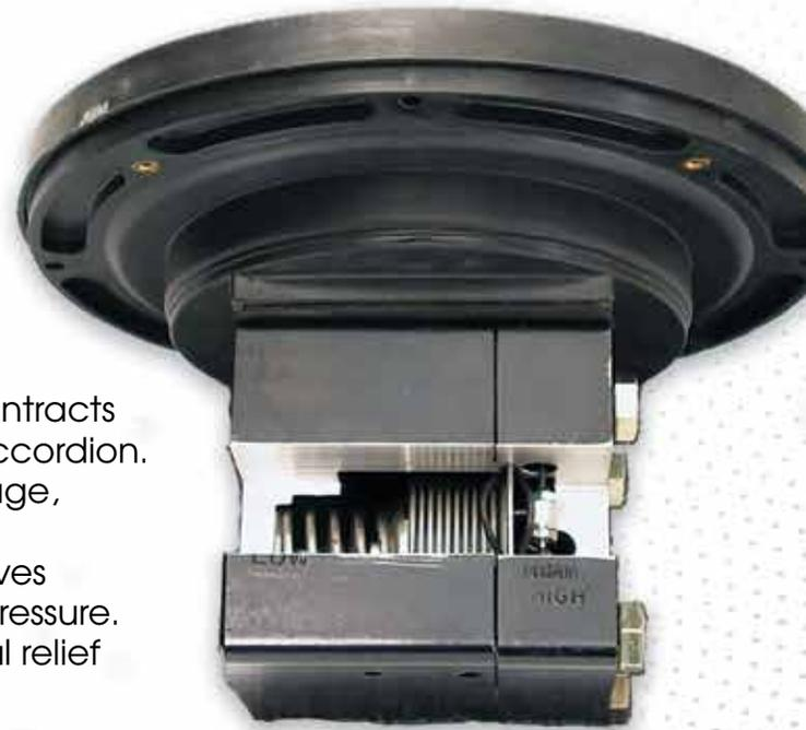
A bellows is a flexible element that expands and contracts when pressure is applied. It operates similar to an accordion. When a bellows is used in a differential pressure gauge, the expansion or contraction of the bellows moves mechanical linkages in the gauge body, which moves the pointer on the dial to display the difference in pressure. Mid-West bellows type gauges feature bi-directional relief valves to provide over-range protection.
