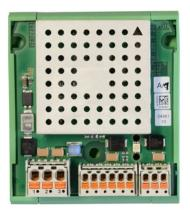
The ADCON A922 Power Adapter was built for customers, who cannot work with solar panels or mains adpaters as power source, be it that the RTU is installed in an area which does not provide enough sunshine, be it that the RTU is inside an electrical control cabinet, where a power source is readily available.
