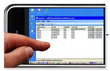
AutoPoll is Sutron software used to schedule periodic downloads of data and/or to collect data-on-demand from multiple Sutron hydromet station loggers and logging sensors, including the following:
