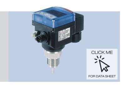
This intelligent sensor / switch with a particularly large display is designed specifically for monitoring limit values or an on/off or continuous control loop. The switching points can be programmed directly via buttons on the display or optionally externally by a PLC via a 4-20 mA standard signal input. In addition, the process value can be transmitted via a 4-20 mA signal to the PLC.
