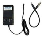
The charger automatically detects the chemistry and the status of each battery within seconds, and selects the charging power and strategy suited best for the resp. battery. A push button provides a controlled refresh cycle, slowly discharging the battery and then fully recharging it again, thus eliminating the negative consequences of memory effect.
