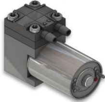
SP 270 EC-LG-L Eccentric Diaphragm Pumps for Liquids Free flow rate: 100 ml/min Max pressure: 14.5 psi / 10.0 m H2O Max suction height dry (priming): -4.35 psi / -300 mbar Max suction height filled: -3.0 m H2O
