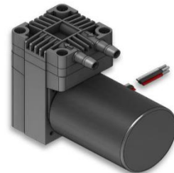
SP 622 EC-BL-L Eccentric Diaphragm Pumps for Liquids Free flow rate: 700 ml/min Max pressure: 21.7 psi / 15.0 m H2O Max suction height dry (priming): -8.7 psi / -600 mbar Max suction height filled: -9.0 m H2O
