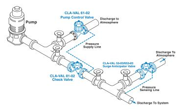
Install Model 61-02 valve as shown. Use a minimum of 1/2" tubing to connect operating pressure connection of the valve to the system side of check valve. Flexible conduit should be used for electrical connections to the solenoid control and the limit switch assembly. A Model 52-02 or 652-03 Surge Anticipator is recommended for power failure and surge protection.
