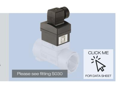
Unique bayonet style flow meter constructed from an SE30 sensor and an S030 flow fitting. Perfect for neutral, solid free liquids. A hall-effect sensor produces a square wave frequency proportional to the flow rate.
