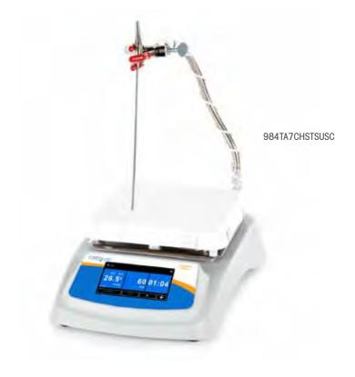
Maximum Temperature Limiting (Plate Over Temperature Limit): Ensures plate temperature will never exceed users programmed set temperature limit, allowing for control of samples with sensitive flash points (heating models).
