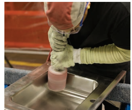
Almost 90 years of experience at forming, welding, trimming and polishing goes into every Elkay sink.
