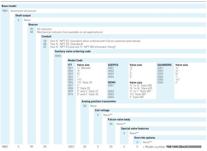
\* Eliminator fitting is  $\frac{1}{2}$ " NPT (M) for the purpose of mounting an aftermarket solenoid valve.
