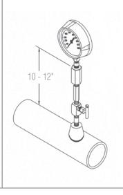
The most streamlined installation results from the use of the Hex HGVS Gauge Valve / Syphon Combination.
