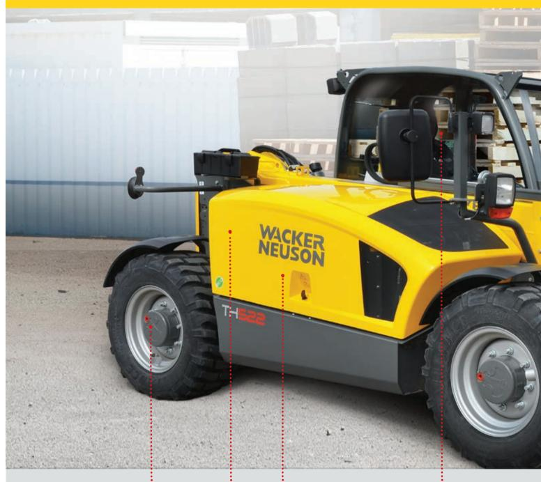
Hydrostatic allwheel drive with an inching brake pedal provides maximum power, while ample ground clearance and off-road mobility handle varied terrain.
