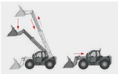
Bucket Mode automatically retracts the bucket when lowering the boom. The ratio of the retraction to lowering movement is designed so that the machine does not go into the overload range, even with maximum payload. The automatic retraction can be overridden with the joystick until reaching the overload limit.
