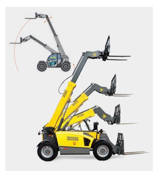
Fork Mode extends and retracts the boom automatically when the operator raises the arm, in order to keep the load in a vertical plane. This is ideal for shelf loading and similar tasks. By operating similar to a forklift, the operator does not have to adjust (extend/retract) the boom while loading. In addition, a digital display monitors the load on the machine and both visually and audibly alerts the operator that the machine is at-risk of tipping.
