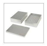
Recommended sealing temperature and time for all PP microplates is 175°C and 3 seconds. Time and temperature can vary depending upon combination of film and microplates being utilized.
