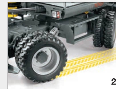
All-wheel steering for a small turning radius.
