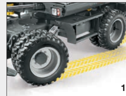
Front wheel steering for fast driving on the road.
