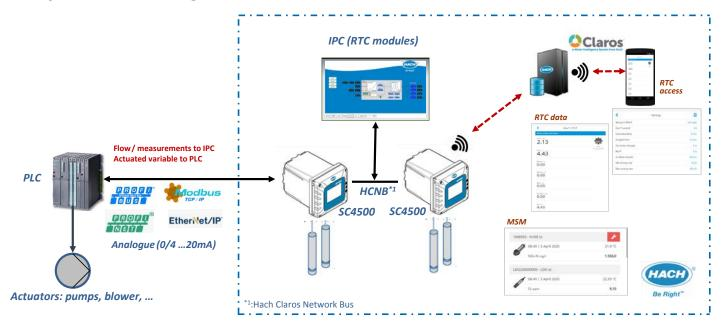
RTC modules are installed on an industrial PC. The site PLC communicates with the SC1000 via PROFIBUS, MODBUS TCP/IP or analogue (0/4...20 mA). The data exchange between the IPC (on which the RTC modules are installed) and the SC1000 takes place via an internal RTC communication card.
