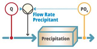
Precipitant has to be well mixed with the wastewater stream before the measurement sample is taken. The application of this technique is not specifically limited by hydraulic retention time. As the precipitation chemicals are highly acidic they "equalize" rapidly across a settlement or aeration phase (just as pH adjustment rapidly effects the whole tank volume).
