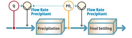
primary dosing point, the secondary open loop control can compensate to ensure breakthrough of orthophosphate does not occur. The ability to choose the balance of phosphorus removal across to dosing points opens up further chemical efficiency.
