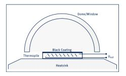
The thermopile output signal is in the order of 10  $\mu$ V (microvolts) per W/m<sup>2</sup> of solar irradiance, so on a sunny day of 1000 W/m<sup>2</sup> the output will be around 10 mV (millivolts). This means that in order to see changes of 1 W/m<sup>2</sup> the data logger input must be able to accurately measure 10  $\mu$ V, this generally means a 'scientific' type of logger.
