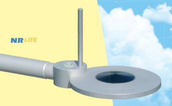
NR Lite is a low cost net radiometer with a Teflon™ coated, weather resistant black conical absorber. A vertical stick prevents birds from affecting the measurement. NR Lite is based on a single differential thermopile sensor and has one output for the total net radiation.
