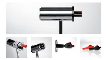
CA2 is based on the same type of thermopile detector as our CMP3 and CMP6 pyranometers. Because it has a limited field of view it can be used to measure the intensity of radiant fluxes coming from a specific location or a specific source.
