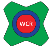
Coolant Water Return
