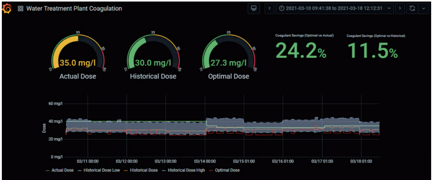
The RTC-COAG software includes powerful trending and visualization tools for real-time visibility of coagulation process performance and results.
