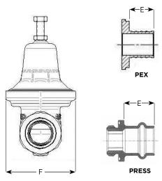
Apollo 36LF Series pressure reducing valves provide automatic control of excessive water pressure and problem supply fluctuations. These models are designed to reduce pressures of up to 300 PSI to a more manageable range.
