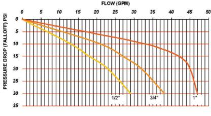
\*Falloff is the difference between the PRV's set pressure and the flowing pressure at any given demand
