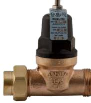
The Apollo 36ELF is designed for residential and commercial applications to protect water supplies from excessive pressure. Excellent flow performance at low pressure drop. The dezincification resistant bronze body and dielectric polymer cage provide maximum corrosion resistance. Designed for easy in-line servicing with simple cartridge removal. They meet ASSE 1003 and CSA B356 standards. They are listed with IAPMO and the city of Los Angeles.
