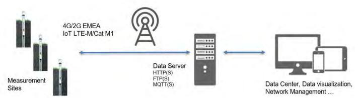
Data is transmitted efficiently in real or near-real time from your monitoring well to your mobile phone or office computer. Transmissions can occur via HTTP(S) and FTP(S) which allows for two-way communication as well as IoT protocol MQTT(S).
