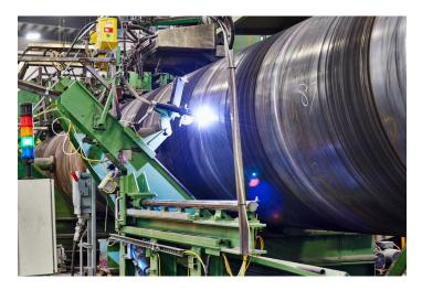
AMERICAN's spiral mills have the capacity to handle coils of steel from 0.1875 inches (4.8 mm) to 1 inch (25.4 mm) in thickness, with yield strengths up to 70,000 psi (482 MPa), to produce high-quality, spiral-welded steel pipe up to 144 inches (3,600 mm) in diameter. This flexibility offers AMERICAN's customers a wide variety of options.
