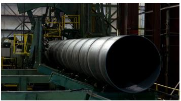
Finished pipe cylinders are moved through the production process by an efficient and ergonomically-friendly pipe handling system.
