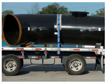
AMERICAN supplies a full line of fittings, including fittings fabricated from spiral-welded pipe cylinders, and/ or cylinders rolled and welded from plate steel up to a thickness of 3 inches (76 mm).
