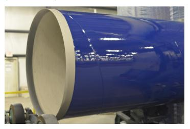
The polyurethane area includes two parallel pipe translators, or conveyors. The first set of translators move the pipe through a pre-heating cabinet to eliminate any moisture on the pipe and elevate the temperature of the pipe for application of the polyurethane. Immediately after the pipe exits the pre-heating cabinet, the pipe enters the blast cabinet where the surface is prepared for the application process.
