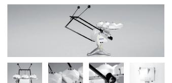
SOLYS2 is a cost-effective and simple sun tracking solution. It does not require a computer and software for installation because the integrated GPS automatically configures location and time data. Multi-colour LEDs indicate the operating status.
