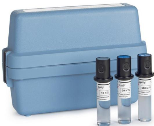
The Stablcal sealed vial standards\* have a long shelf life and can be used for an unlimited number of calibrations and verifications within their expiration date.
