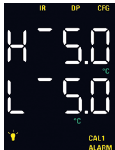
Dew point alarm configuration
