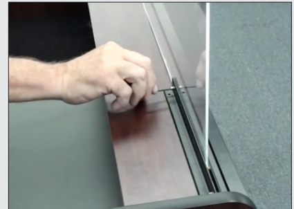
Step 3 - Secure with included set screws
