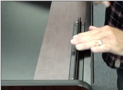
Step 1 - Attach mounting rail(s) with included adhesive
