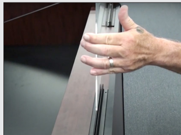
Step 2 - Fit Safety Shield into rail(s)
