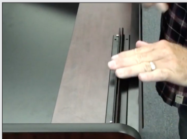
Step 1 - Attach mounting rail(s) with included adhesive
