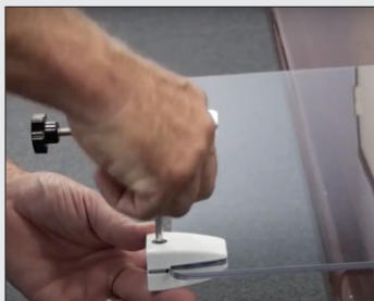
Step 2 - Attach small clamp with hex wrench
