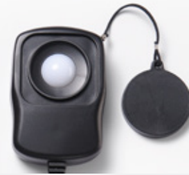
Silicon diode sensor and filter are designed for indoor use.
