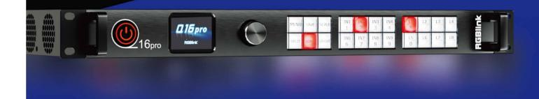
Q16pro Gen2 1U edition supports up to 8 inputs, including HDMI 1.3, SD/HD/3G SDI, HDMI2.0, H.264/265 for 2K and 4K signals. The standard unit comes with 4 HDMI 1.3 outputs and builds with local front control panel and remote control interfaces with RS 232 and ethernet ports. Q16pro is available to be remote controlled by XPOSE or 3rd patry APP / controller by open API.
