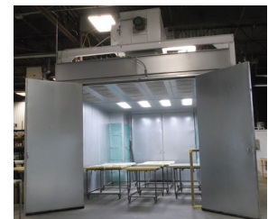
Batch Cure Chamber Interior
