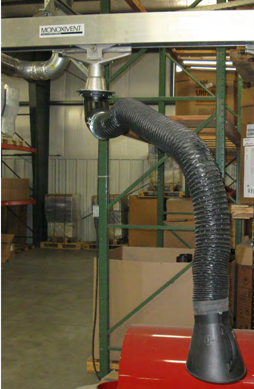
Technorail Welding Arm
