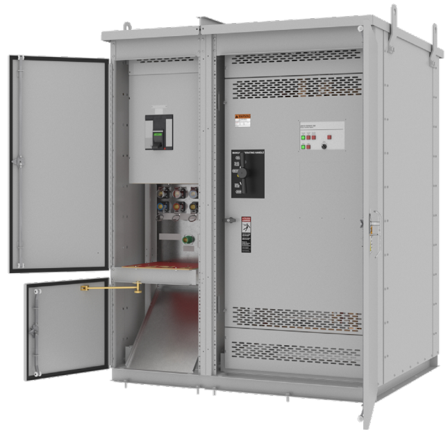
03MGQ Manual Transfer Switch with Quick Connects and a Breaker for a Temporary Genset
