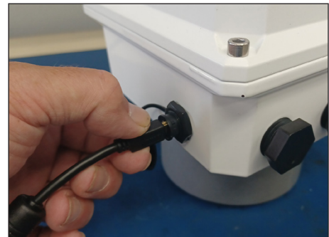
Figure 51. Plug in mini-USB cable
