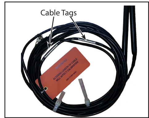
Figure 6. Cables with Cable Tags
