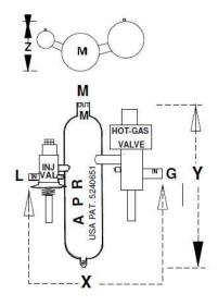
The APR Control Hot Gas Valve should be set to begin opening at approximately 60 PSI ~34°F
