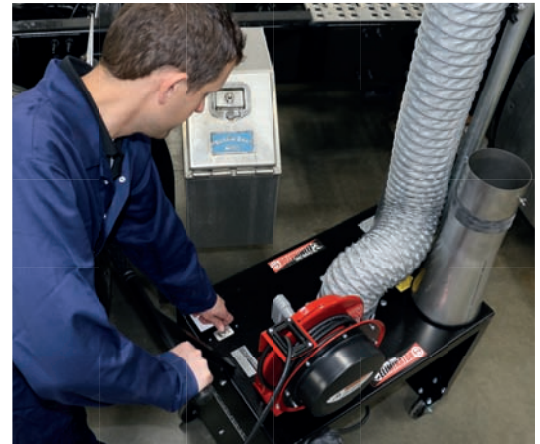
Steel Base Plate Assembly with Radial Blade Blower, Discharge Hose, Power Cord Reel, TCA Adapter
