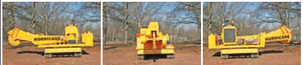
Carlton's patented turret bearing design provides the Hurricane TRX with 360-degree continuous rotation. This gives the Hurricane TRX massive cutting dimensions, allowing the machine to cut a full 19-foot width.
