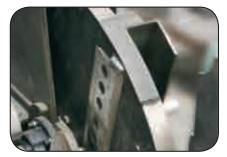
**Precision Ground High Speed** Balanced Chipping Disk. Carlton's chipper disks are perfectly round (no flat spots like competitive chippers) they are also high speed balanced - this combination provides for an extremely smooth chipping action that prolongs bearing and machine life.
