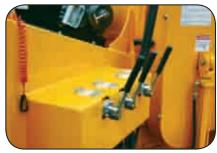
Hydraulic Control Valves are mounted in a heavy duty enclosure to protect them from damage.
