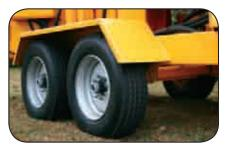
**Two 9000 Pound Capacity Dexter Axles** with electric brakes on both axles make the 2018HD tow great while minimizing tire wear.
