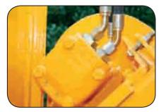
**Super High-Torque Feed Motors** provide the most infeed power of any 18" capacity chipper.
