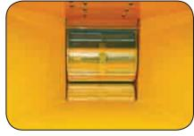
16" Diameter Top Feed Roller aggressively pulls in the material to be chipped. This extra large diameter feed roller climbs over material easily, pulling it into the chipper with no assistance.
