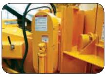
**Dual Lift Cylinders** provide crushing power when necessary and allow easy access to the anvil. Mounting these dual lift cylinders low on the sides allows for a full 360 discharge chute rotation.
