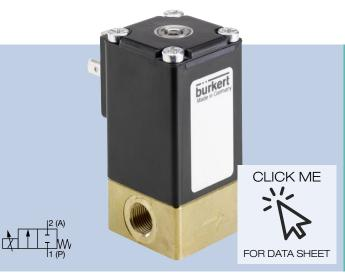
The direct-acting solenoid control valve Type 2873 is used as the regulating unit in control loops. Due to an elastomeric seat seal the valve closes tight (integrated shut-off function), up to the DN specific nominal pressure. The plunger of the valve is assembled frictionless, which leads to an extraordinary adjustment characteristic. This valve is particularly suitable for demanding control tasks (high control range, dry gases, etc.).
