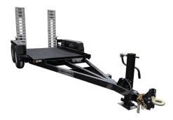
The Dual Axle Steel Trailer is built with two 6,000 lb capacity torsion axles. The trailer can be derated to 9,990 lbs GVWR in order to meet DOT rules & regulations. This heavy duty trailer is equipped with electric, self-adjusting brakes for both axles. Long aluminum ramps make it easy to load our tracked lifts onto the trailer safely & quickly, as well as any other equipment.
