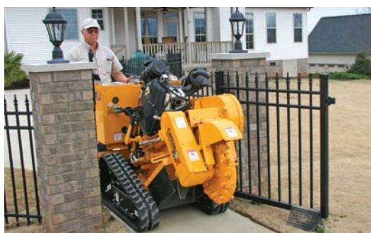
Tracks expand and contract hydraulically from a wide 48 inch stance to gate accessible narrow 35 inch width.
