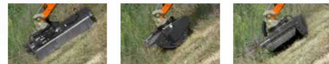
ROTATOR UNIT ROTATOR UNIT FOR 180° ATTACHMENT ROTATION
