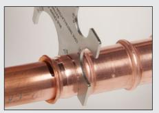
Verify the finished crimp band diameter by using the RLS crimp gauge. Find the proper size slot on the gauge and slide it over the crimp band. It should fit snug, but completely over the band. If not, the fitting must be re-pressed.
