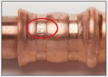
To confirm that the press cycle was completed properly, an RLS witness mark appears within each crimp band (one on each side of the fitting). If the RLS mark is not visible, the fitting must be re-pressed, or removed and replaced.
